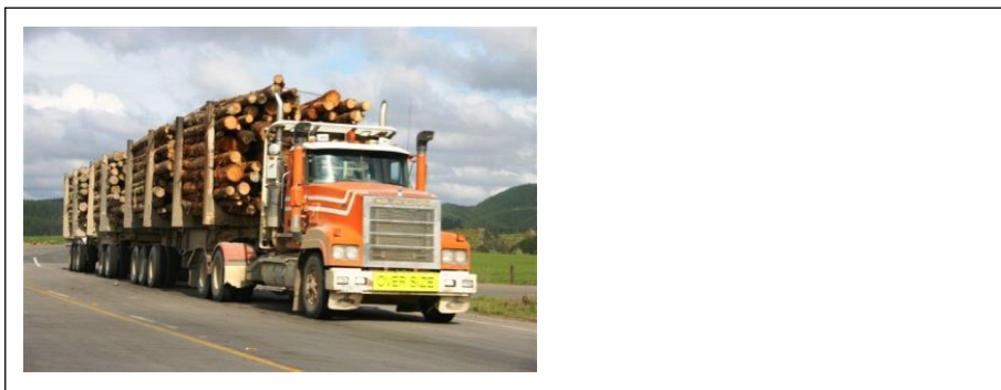
Figure 12. Semi-trailers carrying logs and cars directly without further encapsulation
